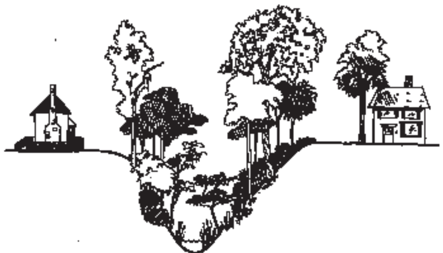
Fig. 12 Build away from crest of the ravine.
